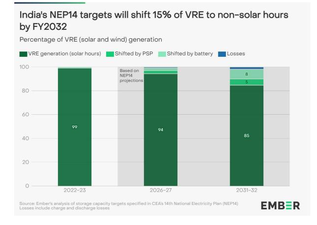
The NEP14 targets to increase India's battery storage capacity to 8.7 GW (4-hr average back up) by Mar-2027 and 47.2 GW (5-hr average back up) by Mar-2032. Pumped storage power plant (PSP) capacity is projected to increase to 7.5 GW by mar-2027 and 26.7 GW by Mar-2032. This planned capacity for storage would be capable of shifting ~6% and 15% of VRE generation to non-solar hours by FY2027 and FY2032 respectively.
